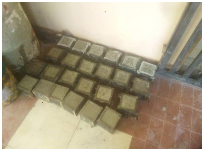
Figure 1: Cast concrete cubes allowed to set for 24 hours.
