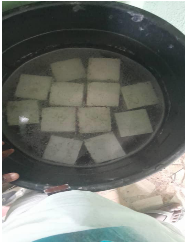
Figure 2: Concrete cubes cured for 7 and 28 days.
